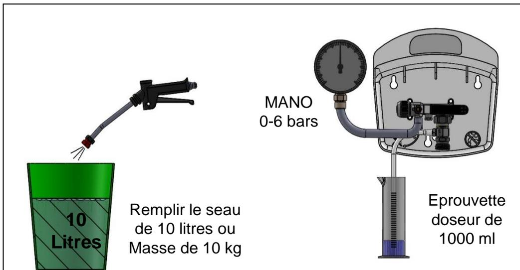
CONTROLE ET DETERMINATION DU VOLUME ASPIRE DANS L'EPROUVETTE
